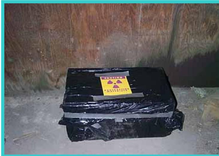
**Figure 3.** Box Containing Depleted Uranium Properly Labeled for Pickup by Red River Army Depot.
