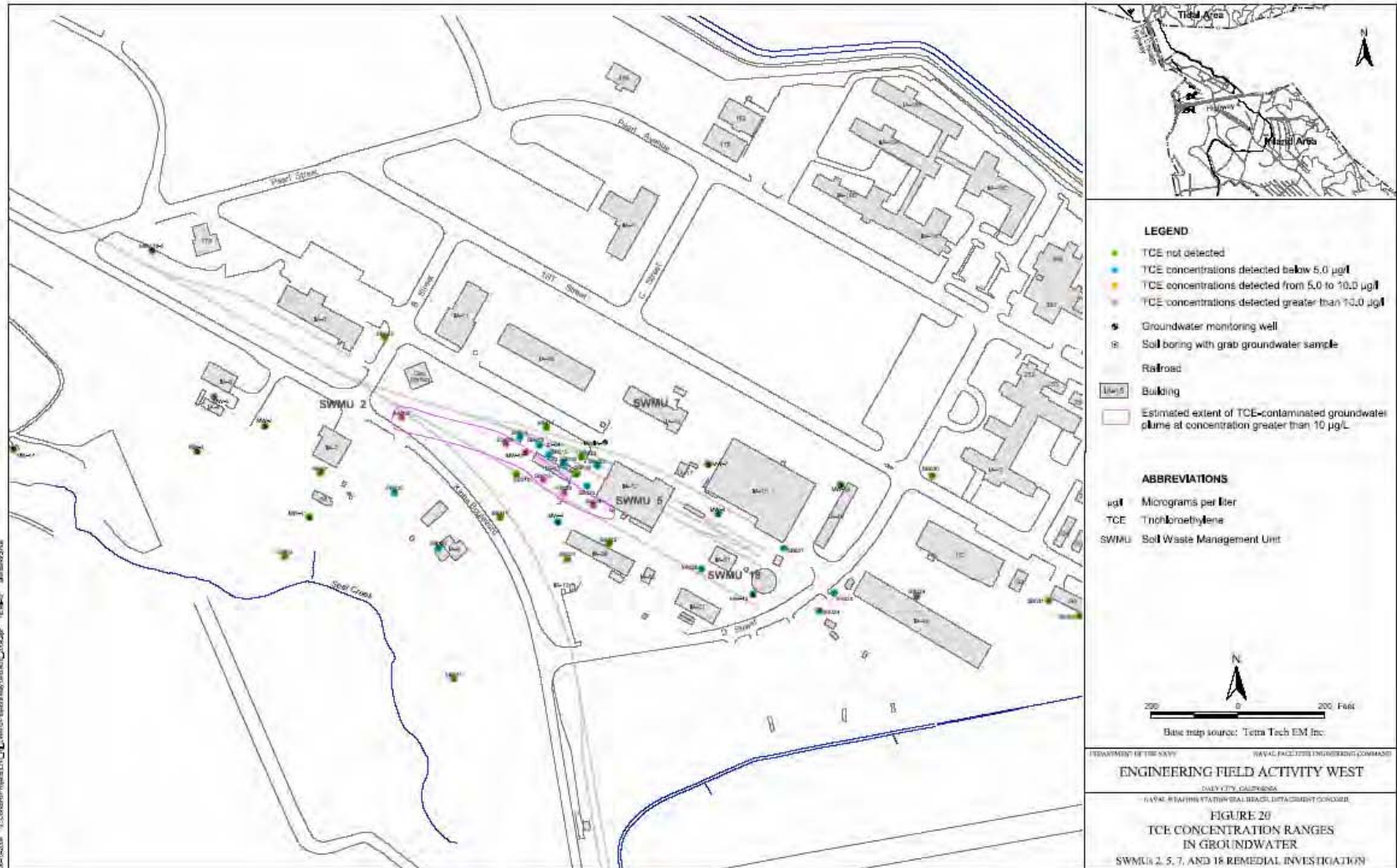
Figure 6. TCE Concentration Ranges in Groundwater
