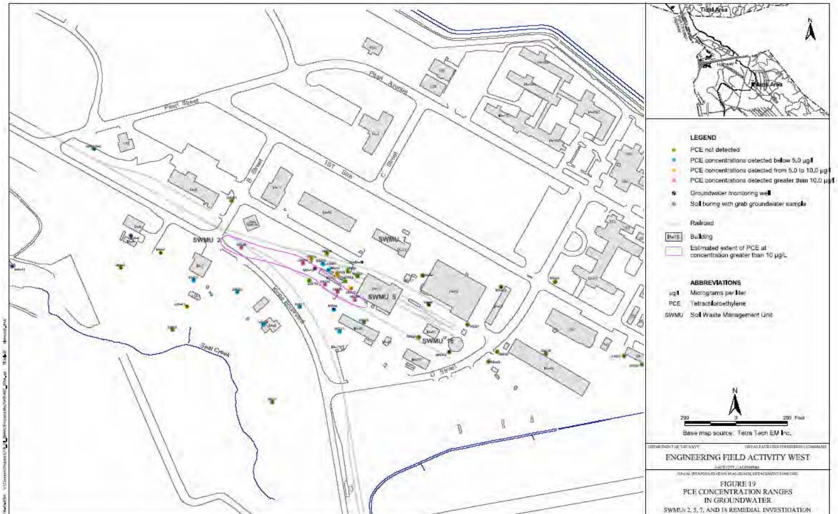
Figure 5. PCE Concentration Ranges in Groundwater
