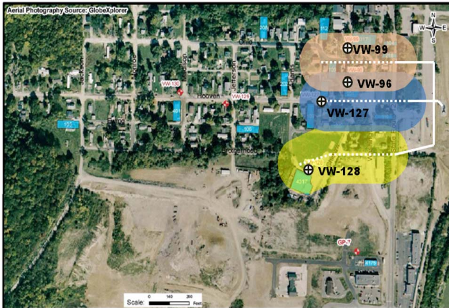
Figure 9 Estimated Zone of Influence of the Horizontal Soil Vapor Extraction (HSVE) System And Vapor Monitoring Well Locations
