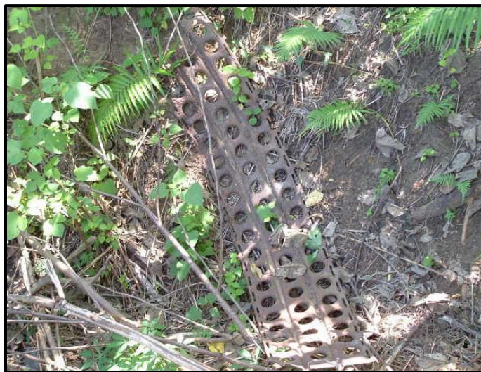
Figure 2: Example of weathered Marston matting
