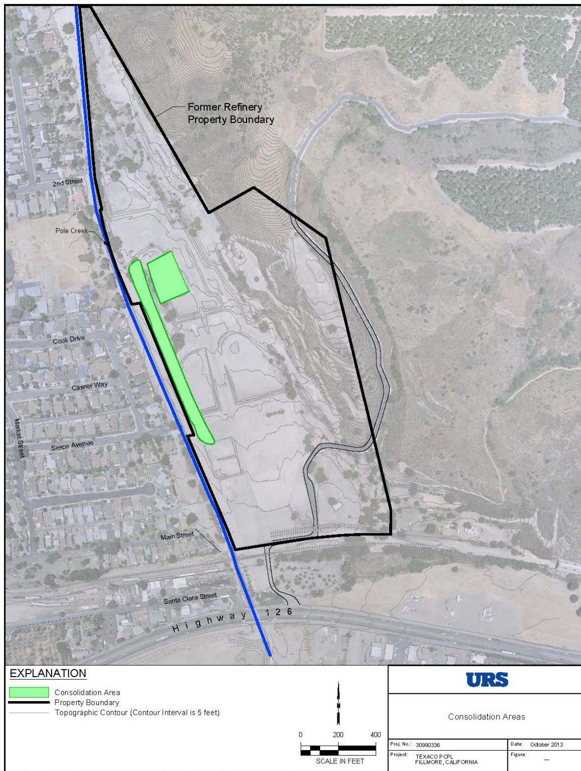
Figure 2. Consolidation Areas where Excavated Soil was Placed During the Clean-up
