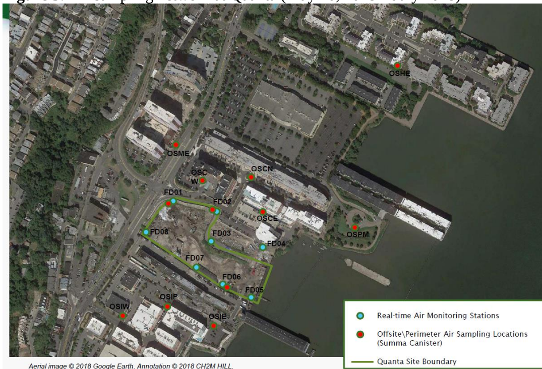
Figure 3: Air sampling network at Quanta (May 10, 2018 – July 2018)
