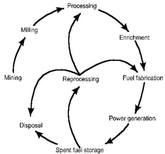
Figure 6-2. Schematic of the Nuclear Fuel Cycle
