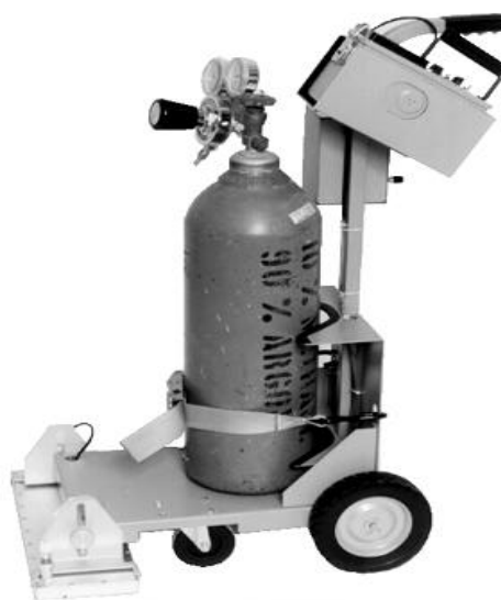
Figure 2-9. Floor Monitor System with Multi-detector Array. (Photo courtesy of Ludlum Measurements, Inc.)
