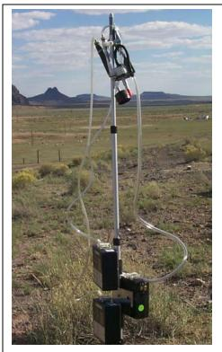
Figure A5. Assembled samplers for dusts and SVOCs
