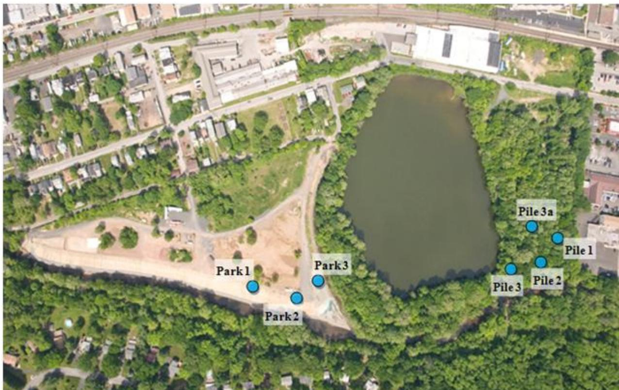
**Figure 3 –** Map of groundwater monitoring well locations at the BoRit asbestos site
