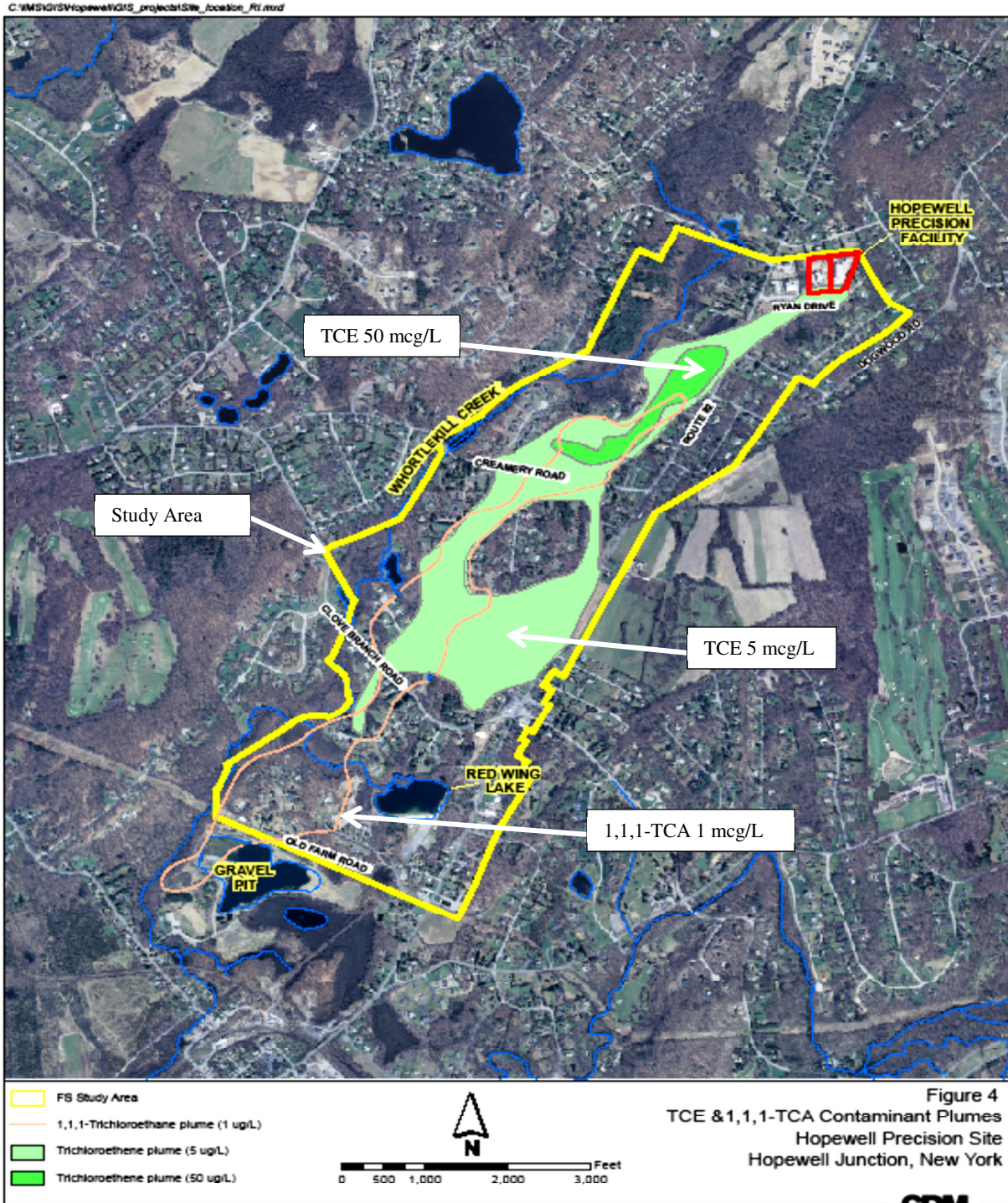
FIGURE 1. SITE LOCATION AND GROUNDWATER PLUME MAP Hopewell Precision Area Groundwater Contamination Site Hopewell Junction, Dutchess County, New York
