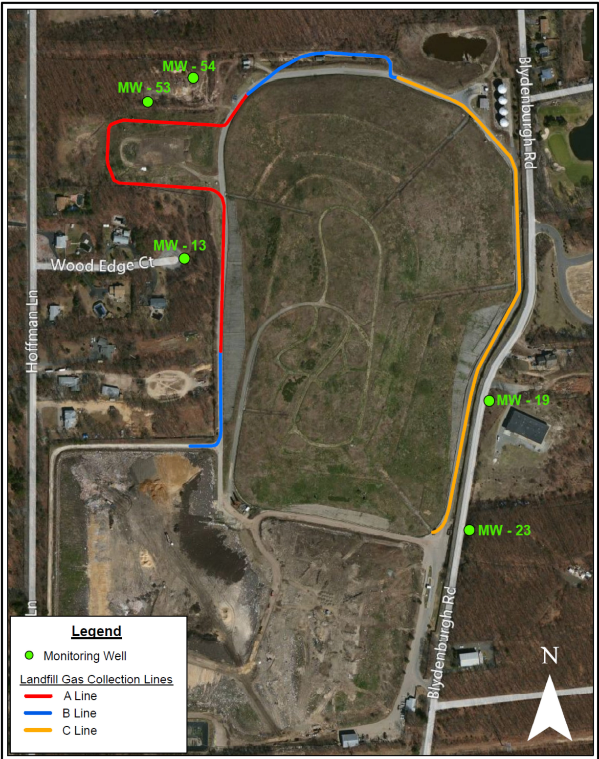
Figure 3 – Landfill Gas Collection System Lines A, B and C and Gas Monitoring Wells
