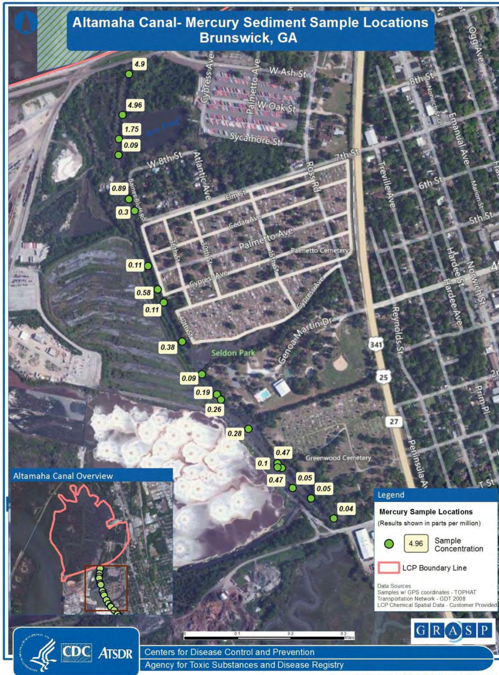
Figure 27. Sampling Locations Showing Concentration of Mercury in Sediment in Altamaha Canal, 2011 Just South of the LCP Chemicals Site.
