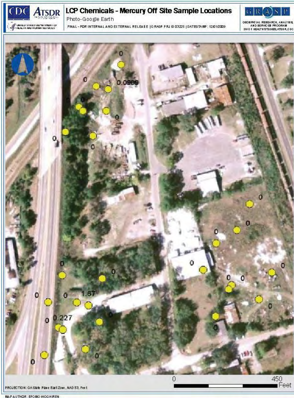
Figure A7. Off-Site Former Tank Farm Area Mercury Sampling Locations and Concentrations
