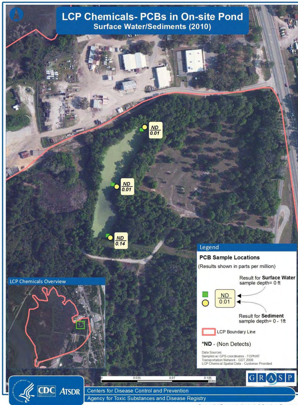
Figure 18. Sampling Locations Showing Concentration of PCBs in Surface Water and Sediment in On-site Pond, 2010
