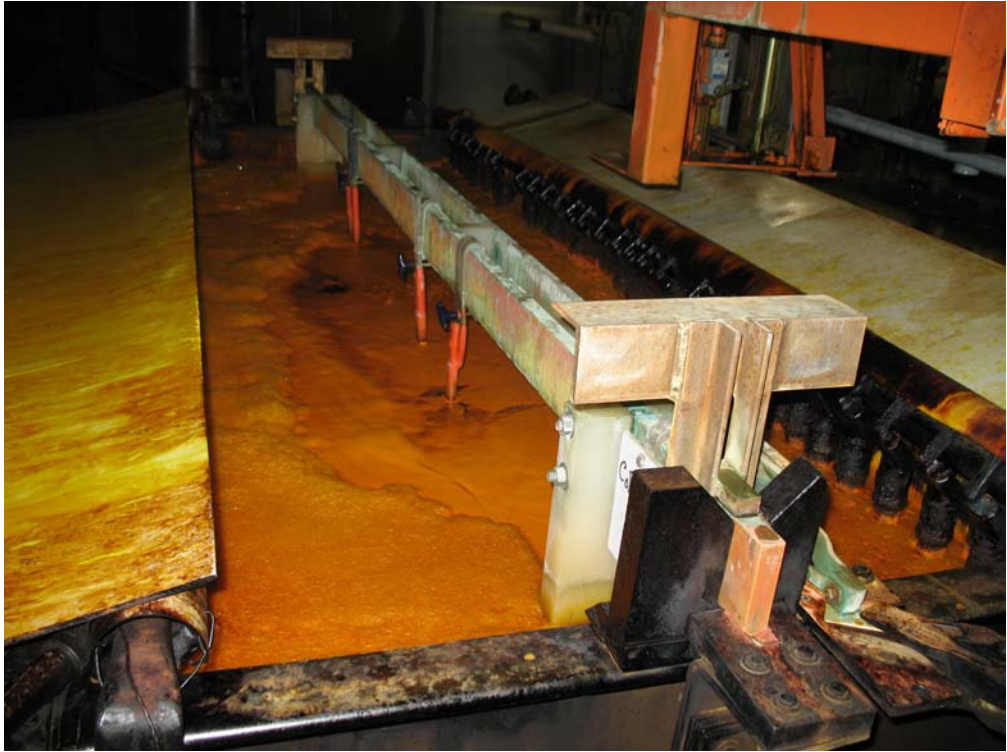
Figure 2 Keystone Automotive Chrome Plating Tank
