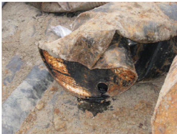
Figure 4: Crushed drum containing some tar
