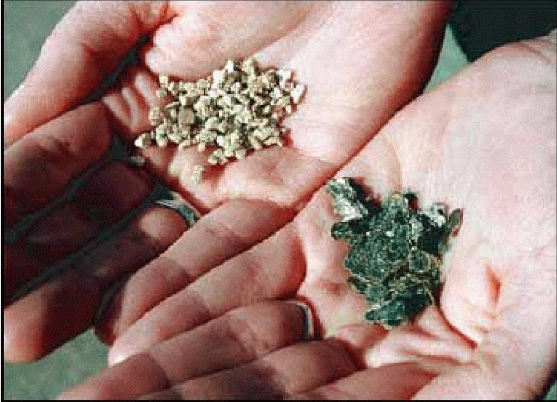
**Figure 3.** Photograph of vermiculite concentrate (on the right) and exfoliated vermiculite (on the left).
