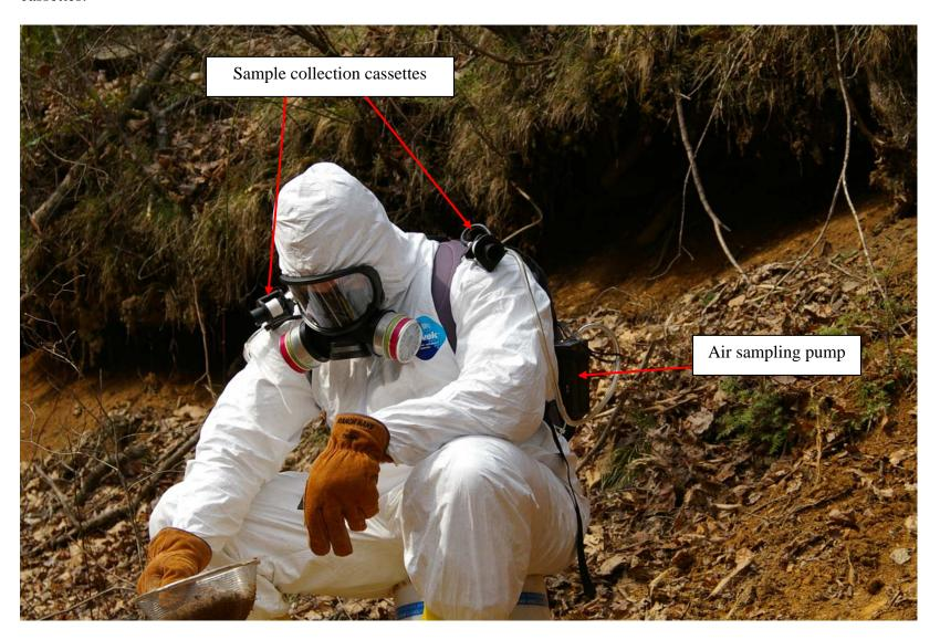
Figure 12. Sapphire Valley Gem Mine site. U.S. EPA activity-based sampling (ABS) event, 2007. Soil shoveling activity. Sampling personnel with breathing zone collection apparatus and upwind and downwind perimeter sample collection apparatus.
