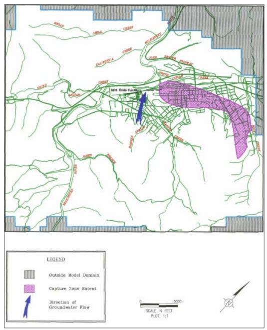
Figure 3. Railroad Well capture zone analysis for 1000 gpm.
